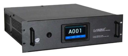
**DRIVENET 832 POWER 24V** is the most advanced rack-mountable, 100-240 Vac 50-60 Hz, power supply / controller unit in DTS range. The unit has been developed to power the DIVE 12 FC LED projector by DTS, working in underwater installations - such as swimming pools - where safety regulations request 24 V DC max voltage. DRIVENET 832 POWER 24 V introduces a series of cutting edge features:
