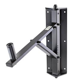
The swivelling and tiltable wall mount holds your speaker at the angle you want. The mount has 11 different tilt settings moving through 22°. The swivel is adjustable to any angle. The patented expanding mandrel for loud speakers with cabinet interiors of diameter from 35 to 37 mm is tightened with a key for a non-wobble and low-resonance speaker fit.
